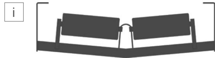
Rigid frame V return roller trains the return belt, adds benefit when carrying more capacities. It's produced with inclination degree of 5°,10°and 15°.
