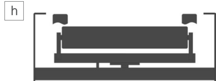
Self-aligning return roller automatically trains the belt return and protects edges from damage cause by belt misalignment.
