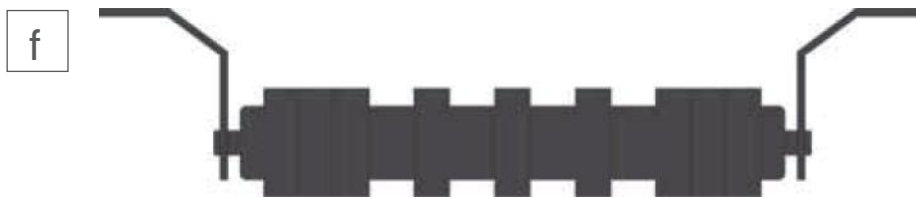
Rubber Disc Return roller used when wet, sticky material tends to cling to the belt. Also used to avoid corrosion .It 's produced in NR or SBR.
